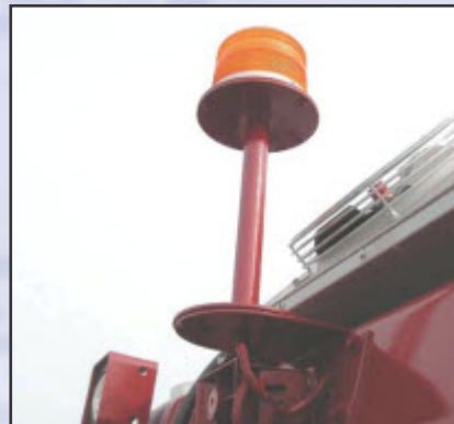
Key-switch actuated amber strobe light; Forward and reverse motion alarms standard
