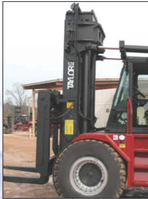
Optional full width fork positioning and optional side shift carriage in variable widths
