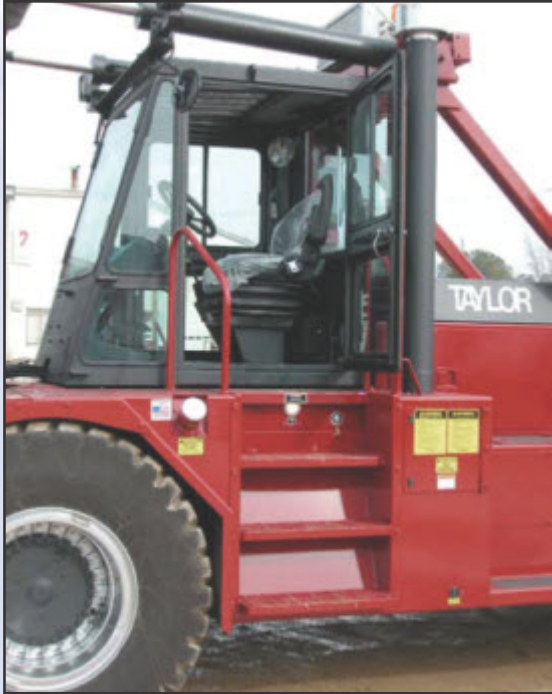
Anti-slip steps and handrails for 3-point mounting and dismounting
