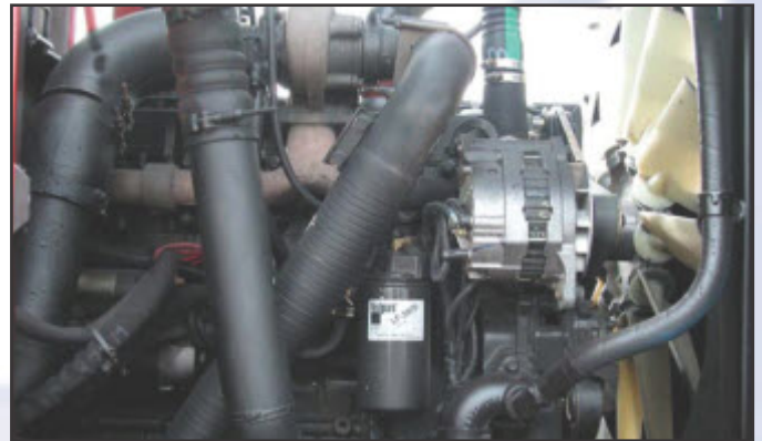
Cummins QSB5.9-C230, 6-cylinder turbocharged engine
