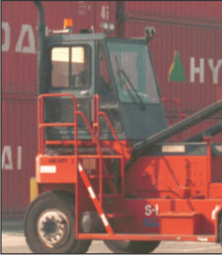
Anti-slip steps and handrails for 3-point mounting and dismounting (meets new proposed ANSI B56.1 standard)
